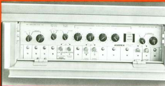
Video signal system controls behind protective flip-down panel... permit compensation for improperly recorded tapes.
