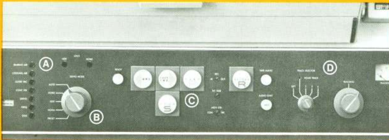
Logically arranged panel features: (A) full protection at-a-glance with meaningful CAUTION, OK and WARNING lights... plus other fail-safe features, (B) complete front panel servo mode control, (C) centralized, interlocked controls for convenient and error-free operation, (D) front panel control and meter indication of all four tracking modes.
