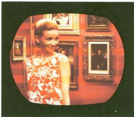
Auto-Chroma "out-of-circuit" during replay of tape; case of chroma banding.
