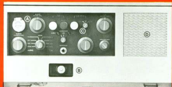
New, audio/cue system has: (A) "spot erase" feature, (B) built-in dynamic mike, (C) switchable cue tone oscillator, (D) built-in speaker plus high-fidelity output for external speaker.
