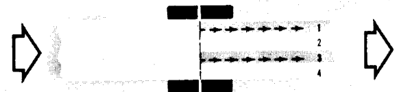
In 4-track STEREO RECORDINGS, the two stereo channels are recorded on non-adjacent tracks in one direction, (tracks 1 and 3 as shown above) from one end of the reel to the other.
