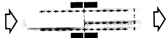
When the end of the second track is reached, the tape is again turned over, and the third track is recorded in the same direction as the original recording. (MONO 2 position)
