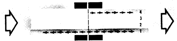
When the end of the reel is reached, the tape is turned over, and the second track is recorded in the opposite direction. (MONO 1 pos.)
