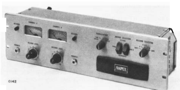
Typical two channel electronic assembly. Ampex Model PR-10-2 professional recorder/reproducer.
