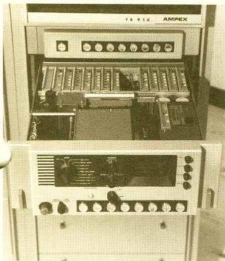
Unit-1 monitor bay of an FR-900A/950. Shown in the "slide-out" position. Plug-in electronics are located inside the drawer.
