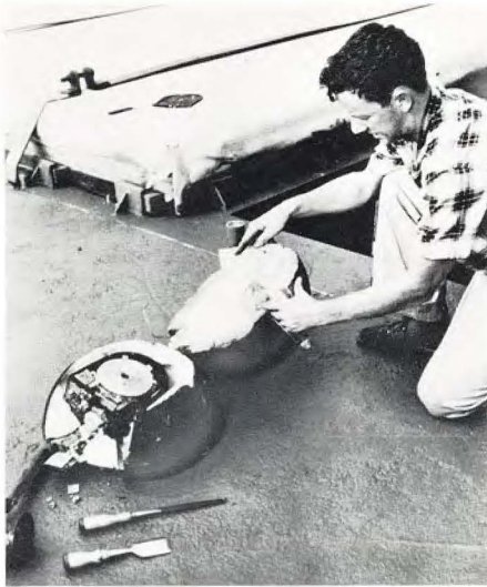
Amper MR-100 Missile Recorders are actively contributing to this nation's missile program. Recorder shown here has been recovered from the sea after being ejected from the nose cone of a test missile.
