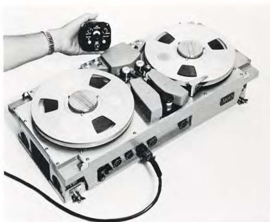
Remote control assembly duplicates all tape-transport controls, plus providing a meter which indicates amount of tape remaining on reel
